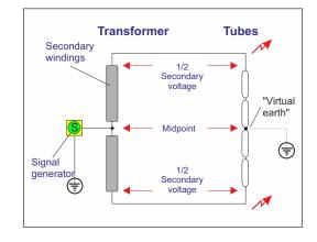
The installation regulation EN 50107 limits the voltage in the high-voltage circuit to a maximum of 5,000 volts to earth. The maximum voltage in the circuit must not exceed 10,000 volts.
