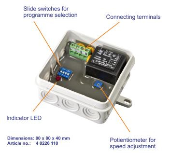
The following flash sequences/programmes can be selected by positioning the four slide switches as indicated:
