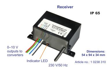
The radio-controlled 4-channel dimmer for 0-10 V can be used to dim or switch up to four output channels separately.
