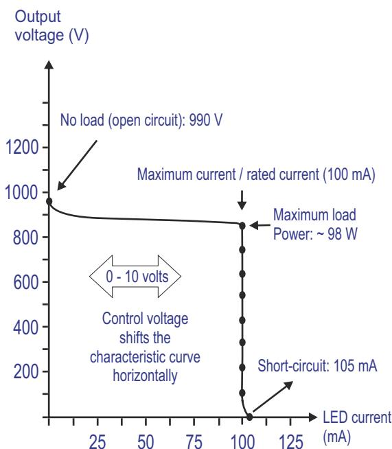
**Maximum loading with 0.4 W power LEDs:**
