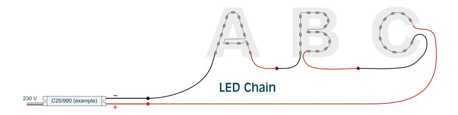
Note: The maximum permitted number of LEDs for the converter must be observed!
