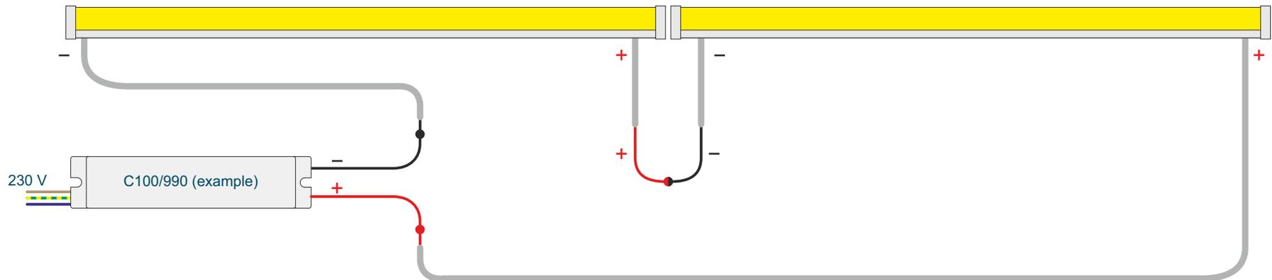
**Caution: The maximum allowed number of LEDs for the converter must be observed!**
