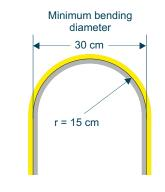
swing~light can be bent horizontally and/or vertically with a minimum radius of 15 cm.
