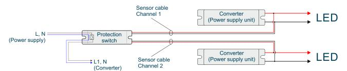
If only one circuit is monitored, the sensor line not in use is short-circuited.
